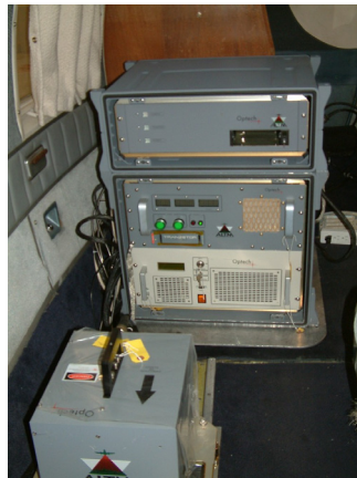
Figure 1: Optech Inc. ALTM 3100 lidar used for surveys
