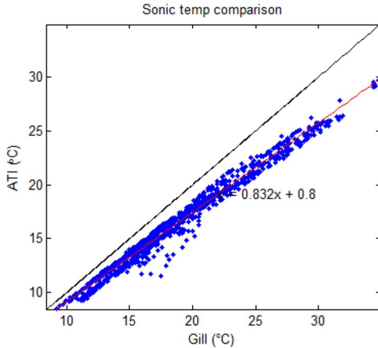
Figure WP3. Comparison of the ATl and Gill sonic virtual temperature responses at West Pond against each other. As expected, the relationship is more linear than that at Sherman due to the more linear response of the Gill at West Pond. The Gill shows about a 17% higher response to temperature than the ATl. The Gill sonic also shows a positive offset from the ATl that grows with higher temperature.
