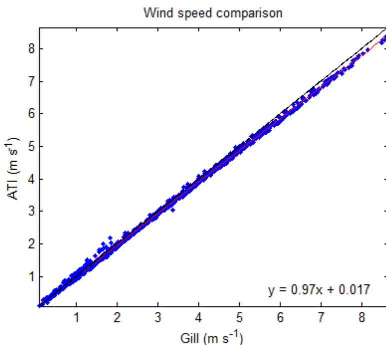
Figure SI-1. Wind speed comparison between the ATl and Gill sonics at Sherman Island. The relationship is linear and almost 1:1, the ATl sonic showing a slightly lower response compared to the Gill.
