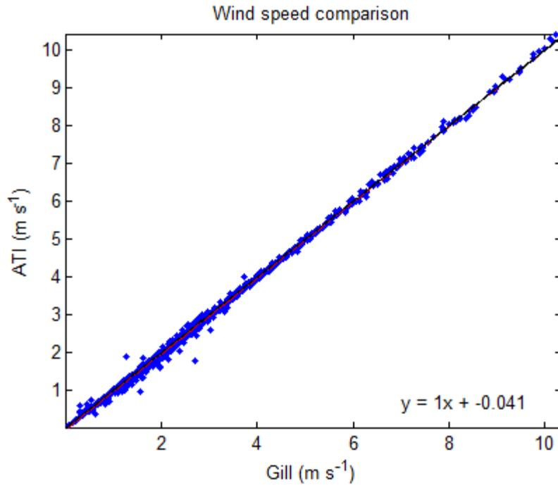
Figure TT-1. Wind speed comparison between the ATI and Gill sonics at Tonzi Ranch. The relationship is linear and 1:1.
