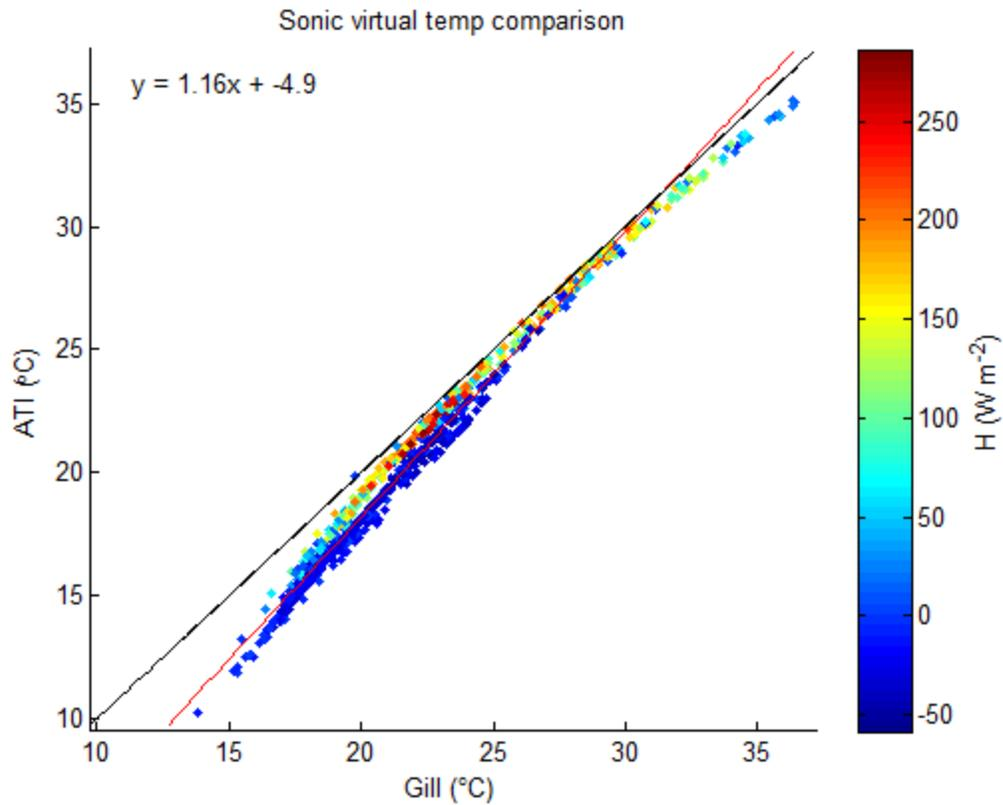
Figure SI-3. Comparison of the ATi and Gill sonic temperature responses at Sherman against each other. As expected, the relationship is curved. The Gill response is lower than the ATi at low temperature, about 1:1 from about 22-27 °C, and higher than the ATi above that range. The Gill sonic shows a positive offset from the ATi that grows at high and low temperature. The Gill's slightly variable response at higher heat flux is also apparent.
