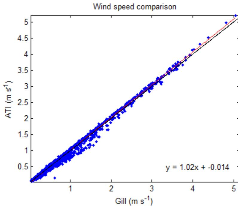
Figure WP-1. Wind speed comparison between the ATI and Gill sonics at West Pond. The relationship is linear and almost 1:1, the ATI sonic showing a slightly higher response compared to the Gill.
