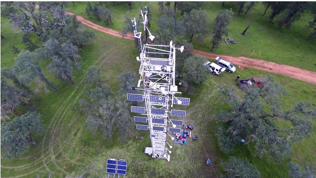
Photo 2. Birds eye view of profile inlet system with PECS EC system visible on back left leg of the tower.
