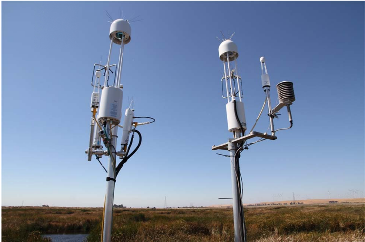
Photograph of eddy covariance sensors during the US-Myb site visit. The left mast held the PECS1 sensors. The right mast included the in situ eddy covariance sensors. The radiation and other sensors were deployed nearby.
