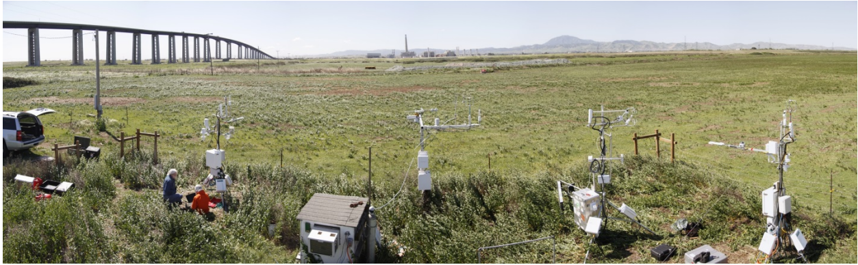
Installed eddy covariance systems at Sherman Island during AmeriFlux intercomparison from left to right (PECS1, in-situ, OSU, PECS2). Photograph orientation is south.
