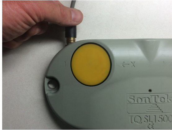
Figure 10. Connecting to SL to the power and communications cable
