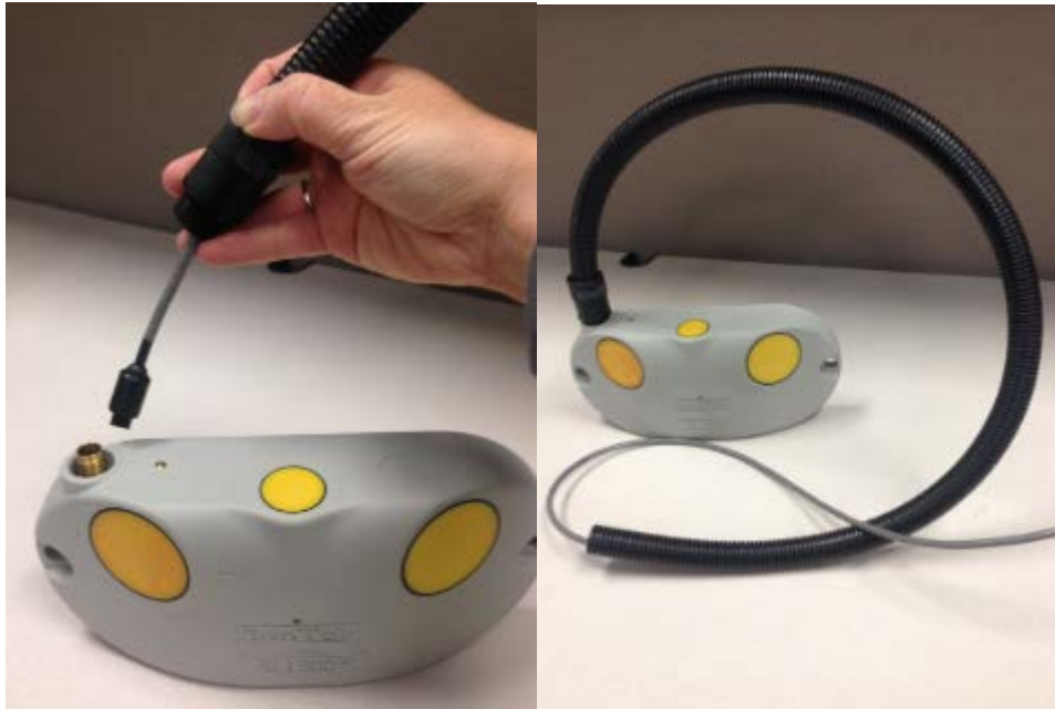
Figure 60. Threads on the cable conduit fitting will screw into threads on the SL1500 housing around the cable connector.
