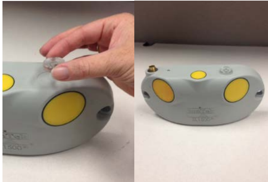
Figure 58. The bubble level provided in the SL toolkit fits into a groove in the housing.
