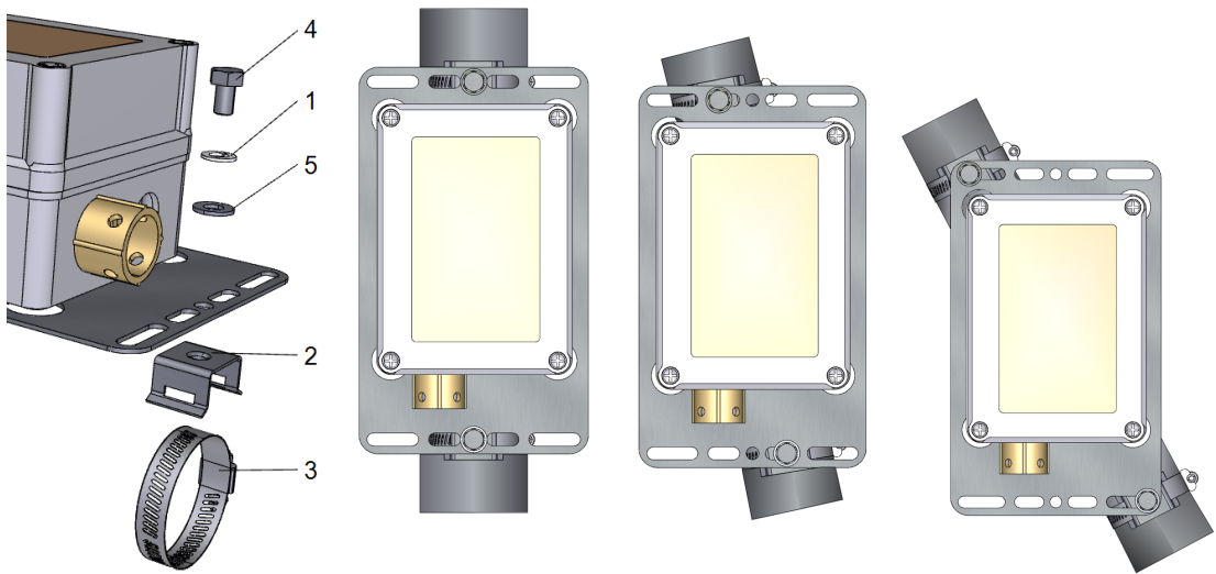
Figure 1-8. Mounting hardware assembly and mounting options.
