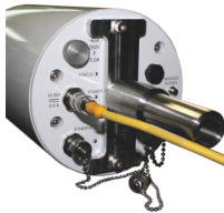
Figure 2-1. Attach the power cable leads to a suitable power supply to turn on the LI-7700.
