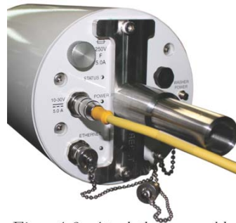
Figure 1-8. Attach the power cable leads to a suitable power supply to turn on the LI-7700.
