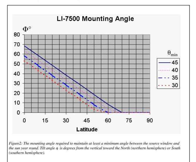
**Caution.** If you are tilting the sensor in (or with) the direction of the mean flow, excessive tilt may introduce anomalies involving flow disturbance and/or heat shedding from the body of the sensor into the optical path.
