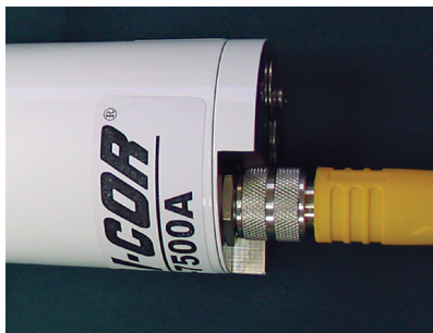
Figure 1-1. Align the connectors and tighten the knurled nut.
