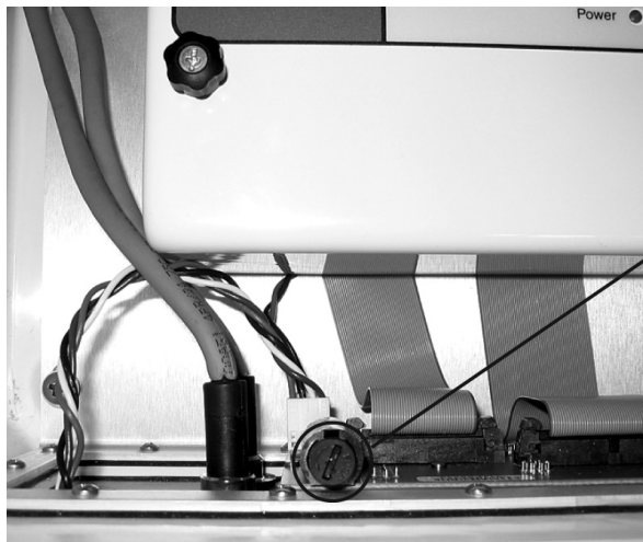
Figure 6-2. LI-7550 fuse location.
