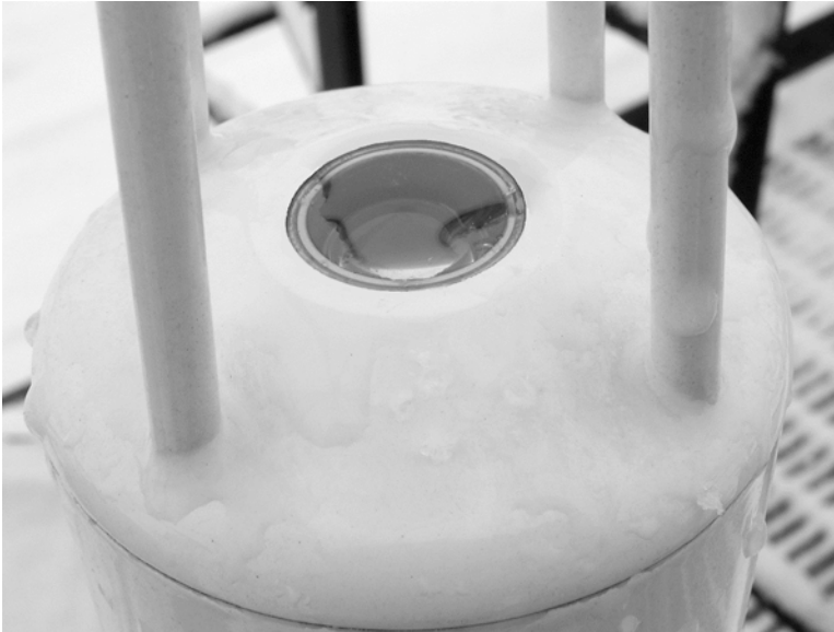
Figure 6-1. Water on the sapphire windows can cause AGC values at or near 100%.
