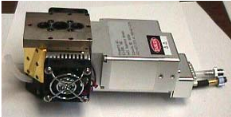
Figure 16-74. The attachment plates mounted on the sensor head.
