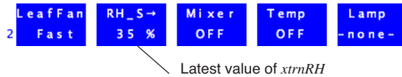
Figure 7-5. When a control has a variable target, the value is updated every 30 seconds. This value is shown on the control key label.
