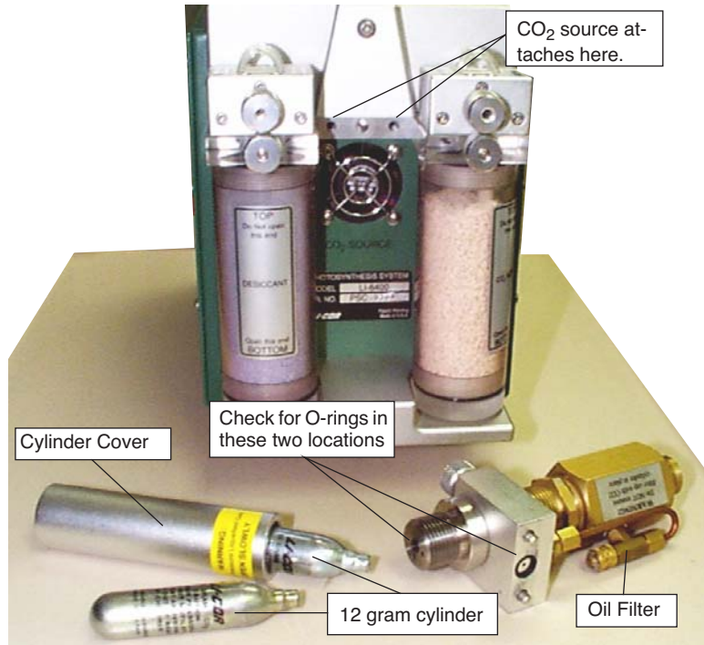
Figure 2-6. Location of external CO 2 source assembly.
