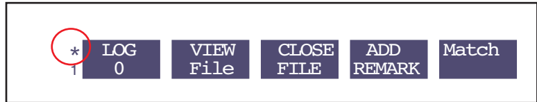
Figure 9-40. An asterisk appears to the left of the function keys while an AutoProgram is active.
