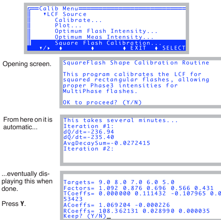
Figure 27-69. Square Flash Calibration. This is an automated routine that is executed from the Calib Menu. This should be run at the beginning of the day and periodically throughout the day if the temperature changes.
