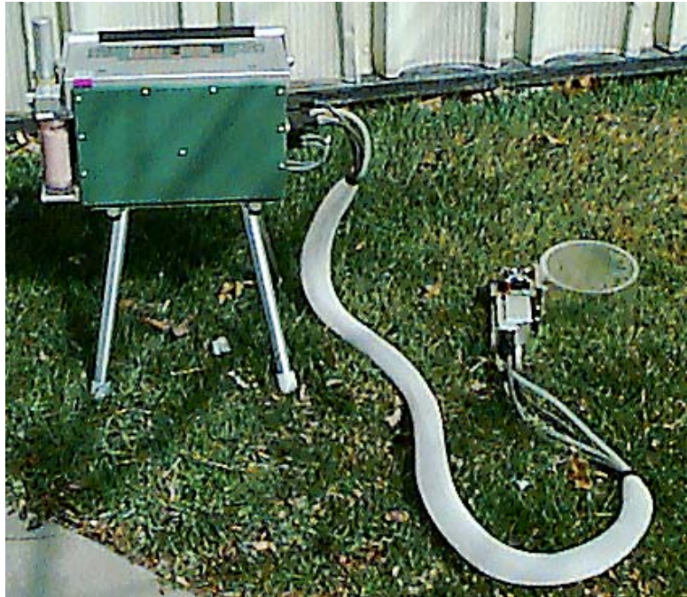
Figure 16-82. Using the custom chamber to measure turf. Note the condensation on the chamber top.
