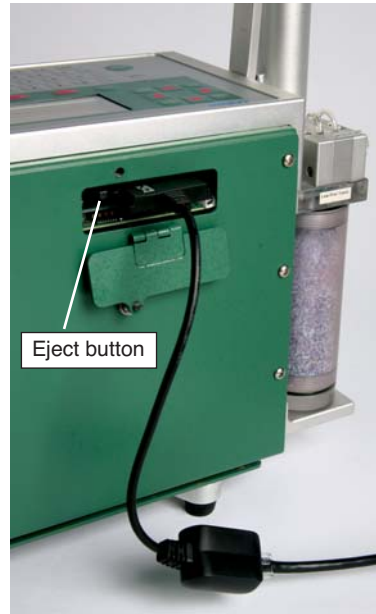
Figure 11-7. Ethernet adapter card inserted in the LI-6400XT expansion slot.
