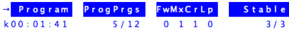
Figure 3-77. The AutoProgram status line includes Program, the time remaining, and ProgPrgs, the current and total program steps.
