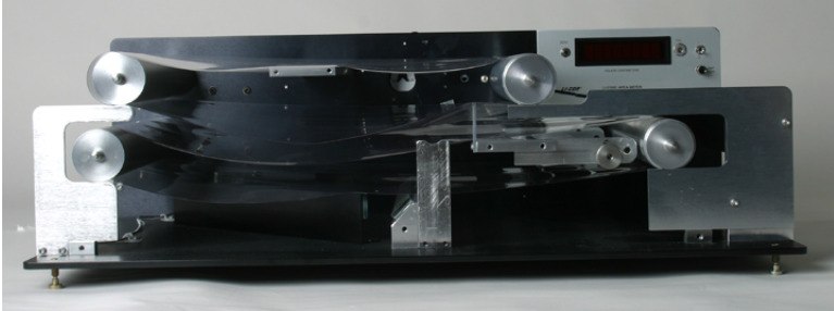
Figure 9. Upper belt rocking idler and lower belt idler removed. To remove the belts, draw them outward.
