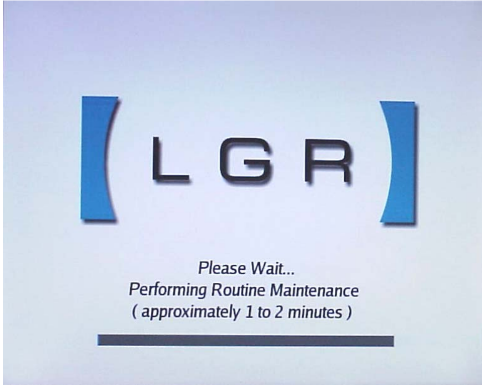
Figure 13: The Routine Maintenance Screen appears during bootup once a month. Normal operation will automatically continue after maintenance is complete. Please do not turn off instrument during maintenance.
