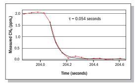
Exponential fit to a portion of the data above yields a 1/e response time of less than 0.1 seconds, sufficient for 10-Hz eddy covariance flux measurements.
