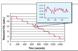
Measurements of methane in calibrated air mixtures over a wide dynamic range. The inset shows the measured methane fluctuations (1 second measurement time) in flowing air.
