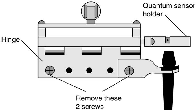
**Figure 2-8.** Remove the 2 screws from the handle hinge.
