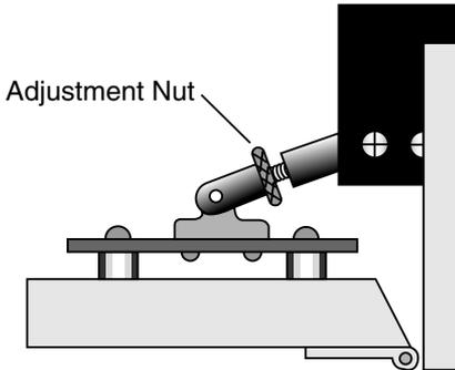
**Figure 2-6.** Turn the adjustment nut clockwise to remove.
