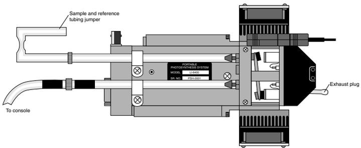
**Figure 5-8.** Hose configuration after changing the tubing to zero the IRGA.
