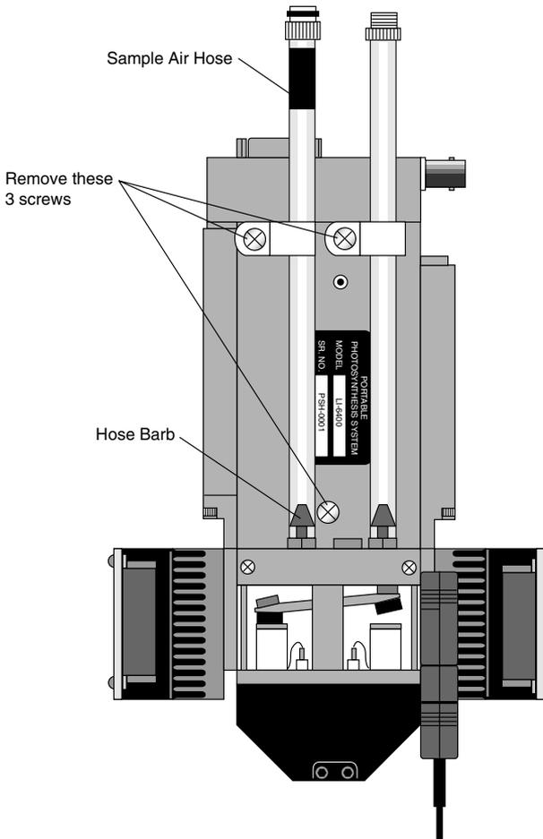
**Figure 2-5.** Remove the 3 Phillips head screws from the bottom of the sensor head.
