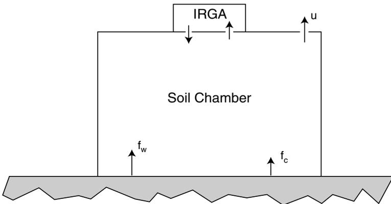
**Figure 6-1.** Schematic of the soil chamber. Soil evaporation  $f_w$  and soil CO<sub>2</sub> flux  $f_c$  add mass to the chamber, which is balanced by a flow  $u$  of air, water, and CO<sub>2</sub> out of the chamber.
