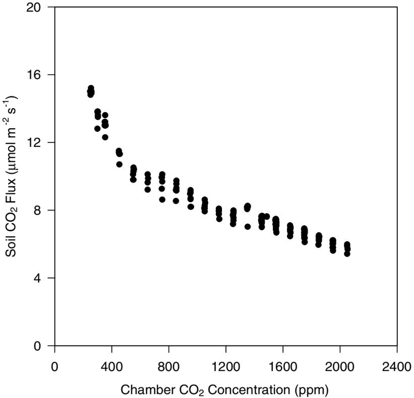
**Figure 1-1.** Soil CO<sub>2</sub> flux rates depend on the chamber CO<sub>2</sub> concentration.
