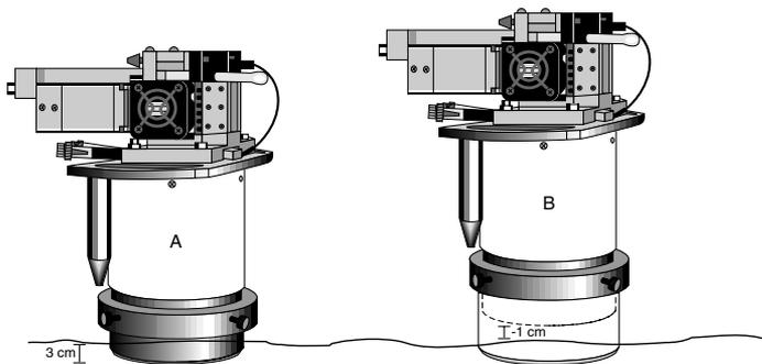
**Figure 4-2.** Measure the insertion depth.
