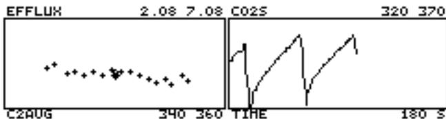
**Figure 4-3.** The real time graphics display "Soil Efflux RTG" will display a strip chart of  $CO_2$  in the sample cell, as well as a plot of soil  $CO_2$  flux as a function of  $CO_2$  for each measurement cycle.
