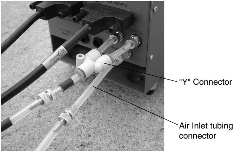
*Figure 4-1. Photo showing plumbing arrangement of 6400-09 and LI-6400.*
