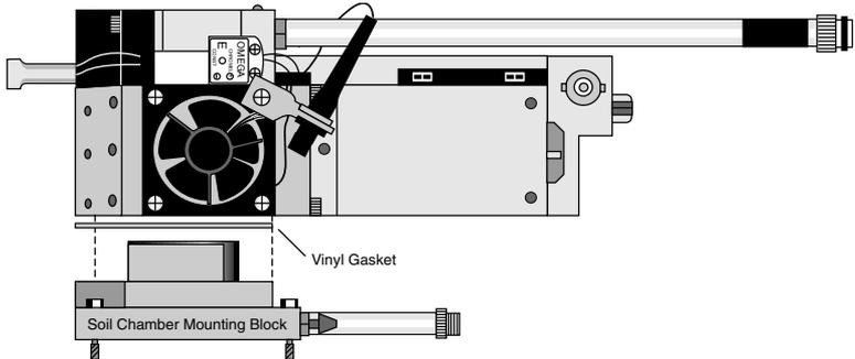
**Figure 2-11.** Attach the mounting block to the sensor head.
