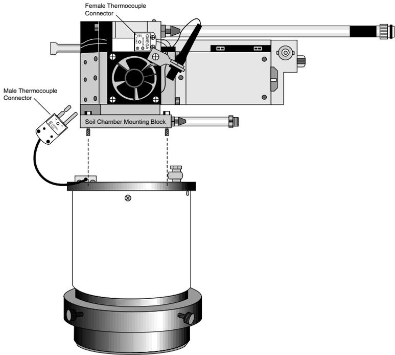
**Figure 2-13.** Attach the 6400-09 body to the mounting block.
