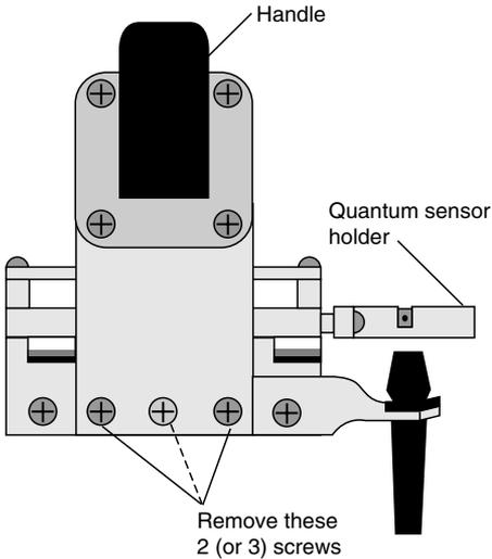
**Figure 2-7.** Remove the screws on the back side of the handle.
