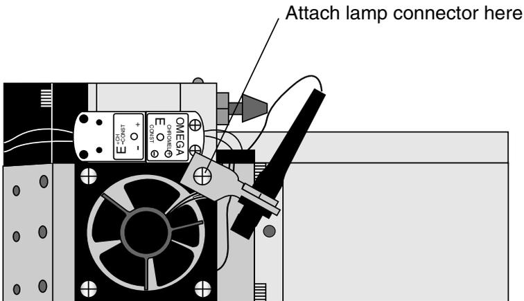
*Figure 2-9. Attach the lamp connector to the fan shroud.*
