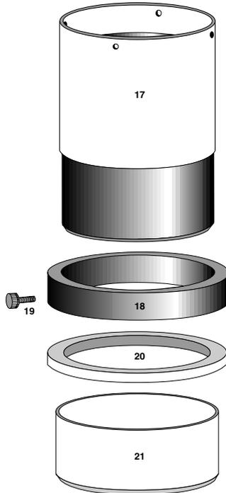
Figure 2-2. Exploded view of soil CO<sub>2</sub> flux chamber.
