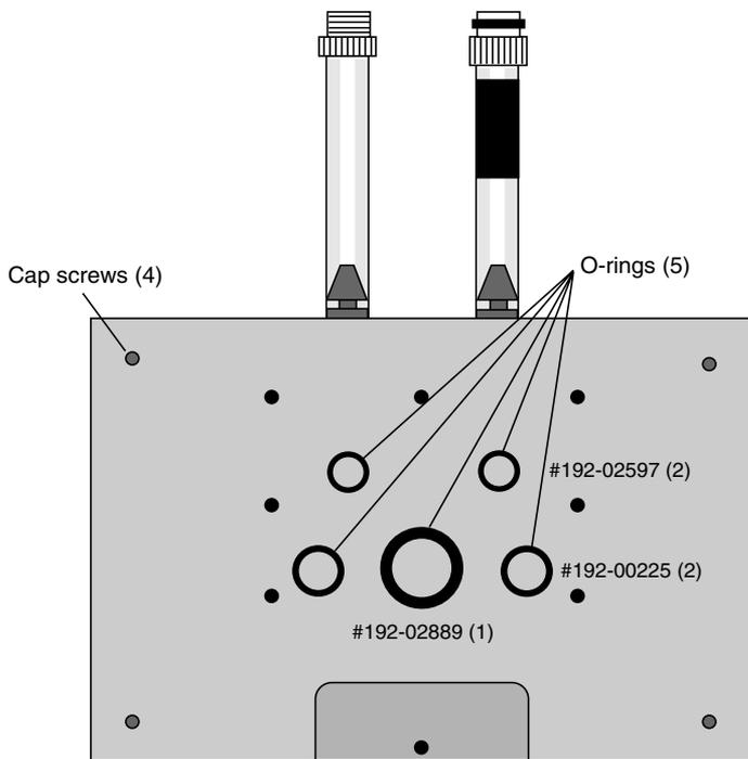
**Figure 2-12.** Location of O-rings and cap screws.
