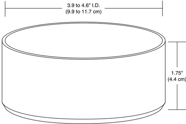
*Figure 5-7. Soil collar dimensions.*
