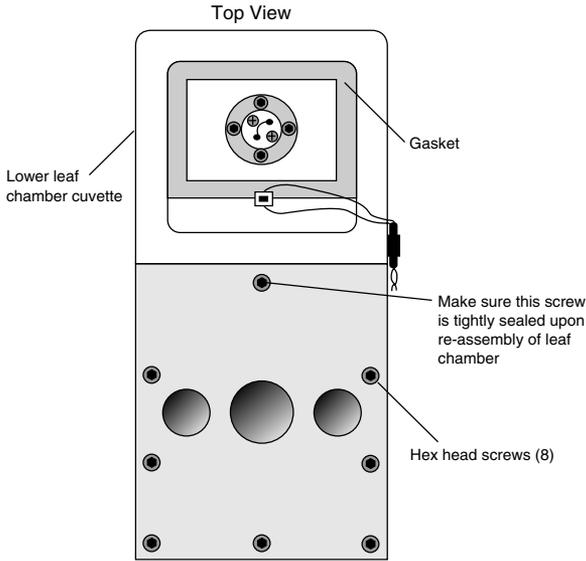
**Figure 2-10.** Remove the 8 hex head cap screws.
