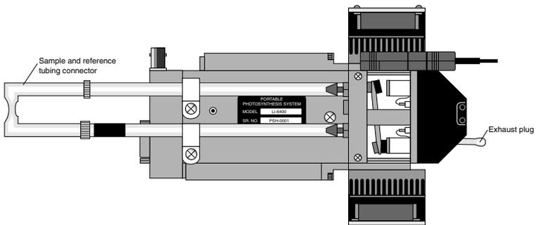
**Figure 2-14.** Insert exhaust plug and sample and reference tube junction as shown.
