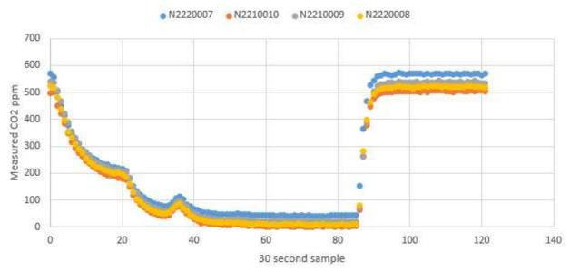
I took the average of 15 reading (samples 70-84) just before the switch to span gas, and the average of 20 sample at the end of the measurements for zero and span readings. The position of the probes in relation to the gas inlet and fan didn't seem to have any relationship to their readings.
