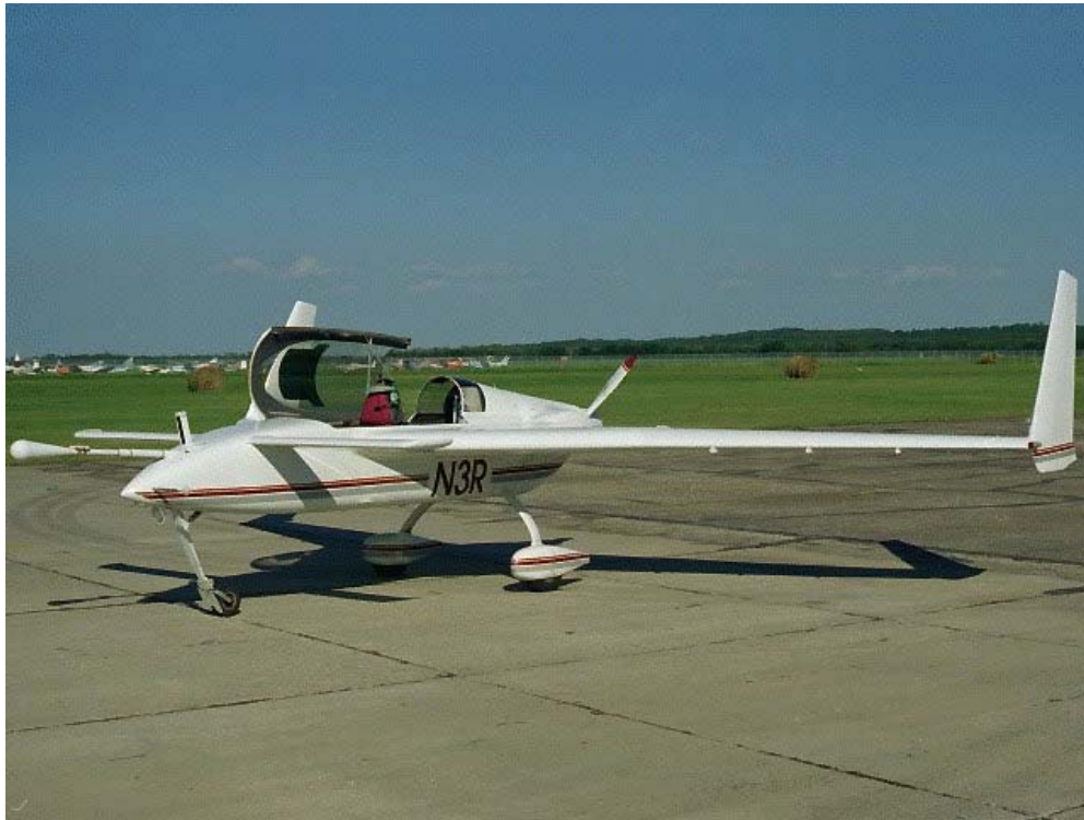
Figure 5 Tim Crawford's Long EZ aircraft instrumented with sensors to measure wind, turbulence, CO 2 , water and heat exchange.
